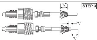
Fan the braid back, as illustrated, and trim it to 3/8". Strip the insulation from the center conductor as shown. **Be careful not to damage the center conductor.**
